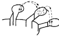
(a) MAGNETIC (INDUCTIVE) COUPLING BETWEEN HOLE AND ITS NEIGHBOURS
