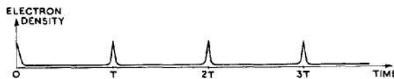
Fig. 414 - Variation of electron density with time in the region of optimum bunching.
