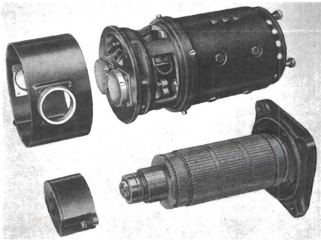
Fig. 2.—Generator, showing brush gear
