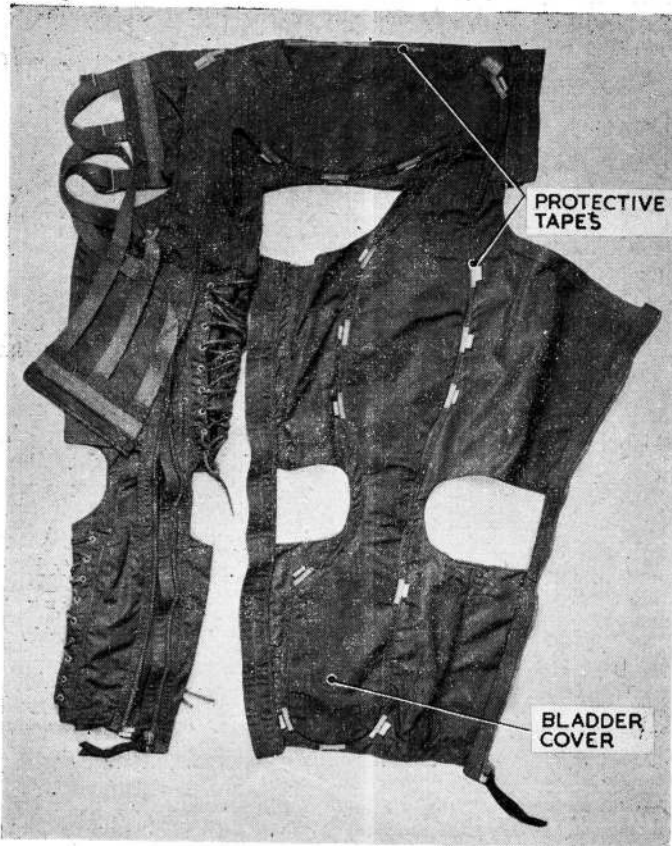
Fig. 5. Internal view of anti-g suit, Mk. 4
