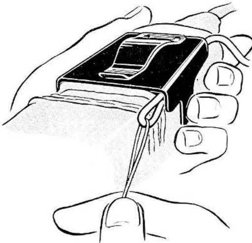
Fig. 4. Connecting the beacon to the battery switch pin: first stage
