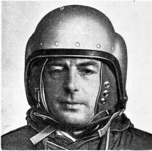
Fig. 8. Protective helmet, Mk. IA, worn over a Type F helmet
