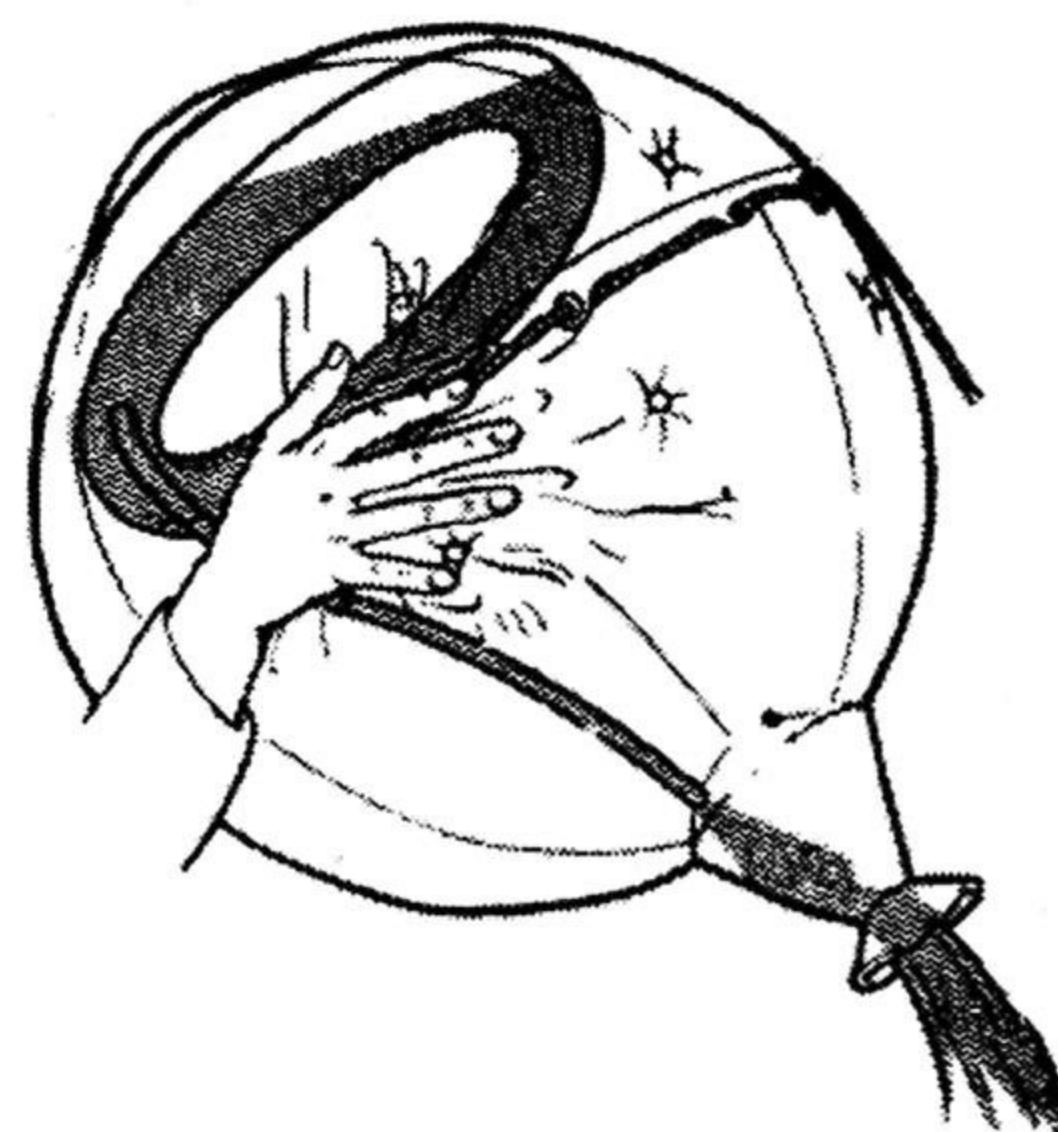
Fig. 16. Emptying sea water and air from Still
