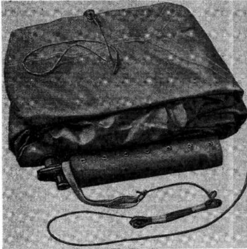
Fig. 8. Third lateral fold ; dinghy ready for stowing in pack
