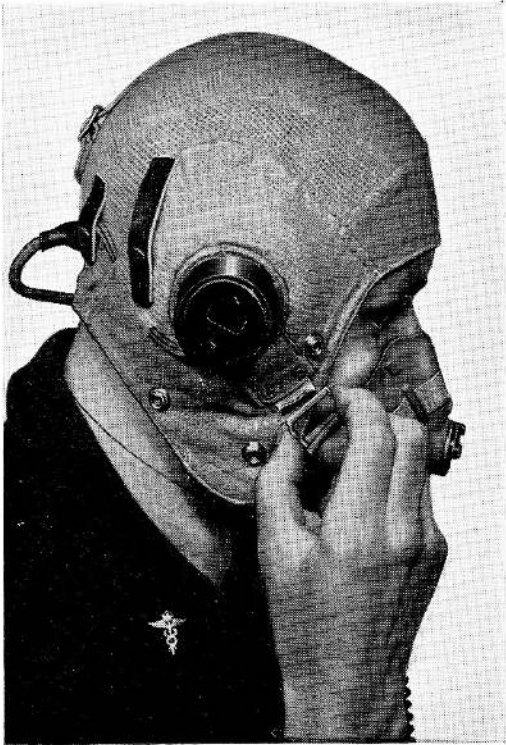
Fig. 9. Attaching the mask to the helmet, stage two
