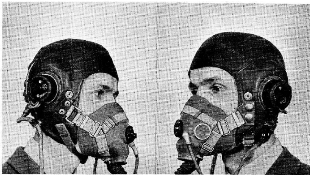
Fig. 3. Strap assembly fitted to mask and helmet
