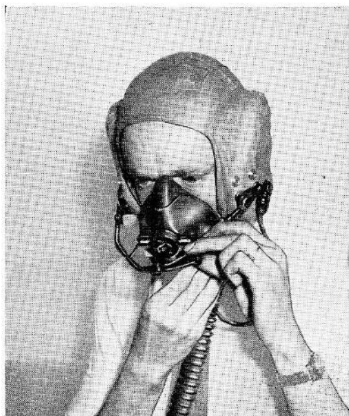
Fig. 10. Snapping the harness into place to locate the outer bow in hooks
