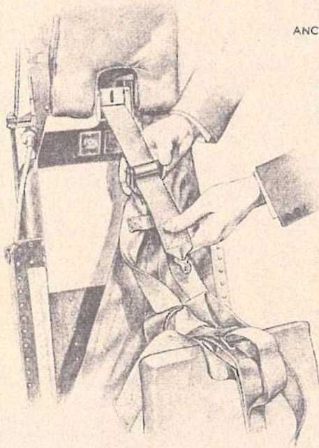
Fig. 4. Installing parachute assembly (Stage 1)
