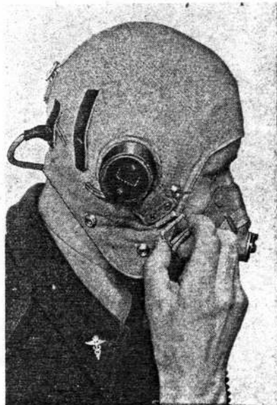
Fig. 4.—View showing the hook on the helmet and ring on the mask, and the correct method of holding the ring by the wings
