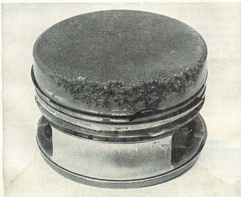
Fig. 2. Effects of Detonation on an Aero-Engine Piston.
