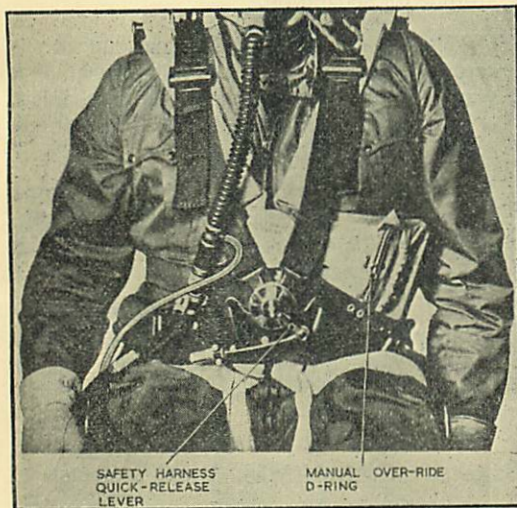
Fig. 9. Manual Override Device (Mks. 2 and 3 Seats)
