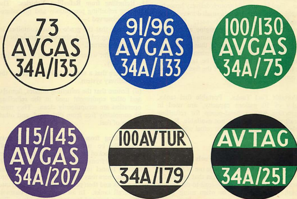
Fig. 1. Fuel Identification Markings Carried on Refuelling Vehicles
