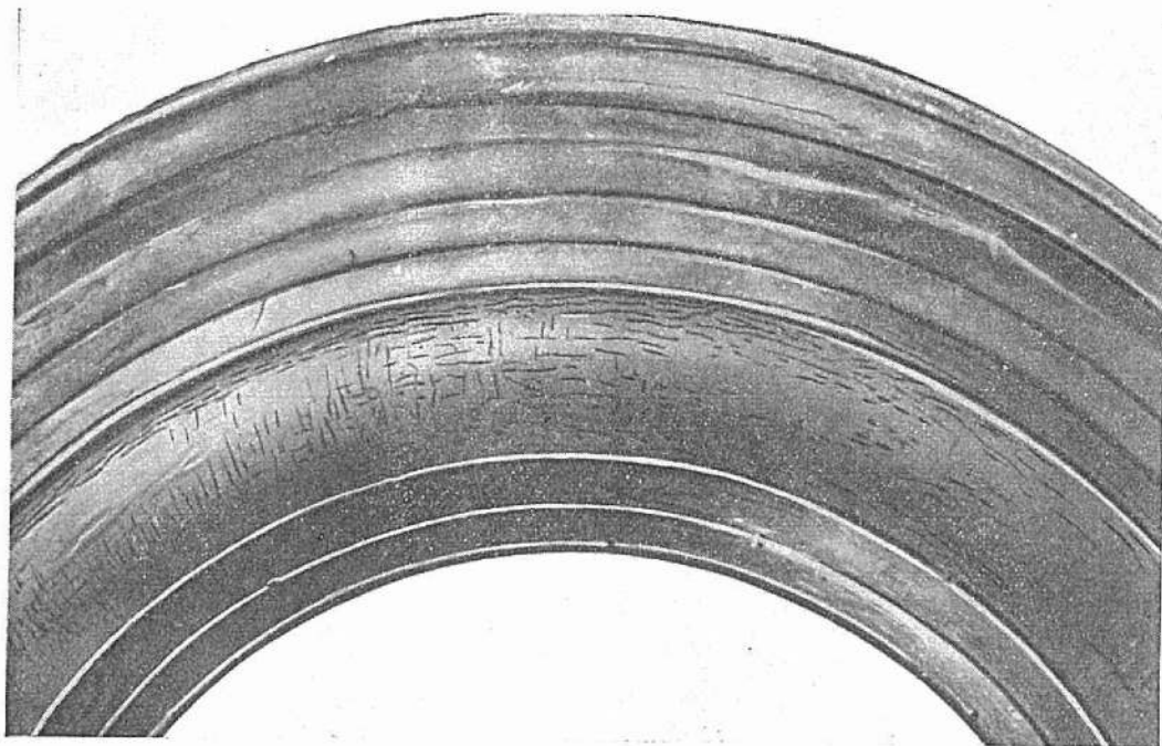
Fig. 11. Cracks in sidewall of cover
