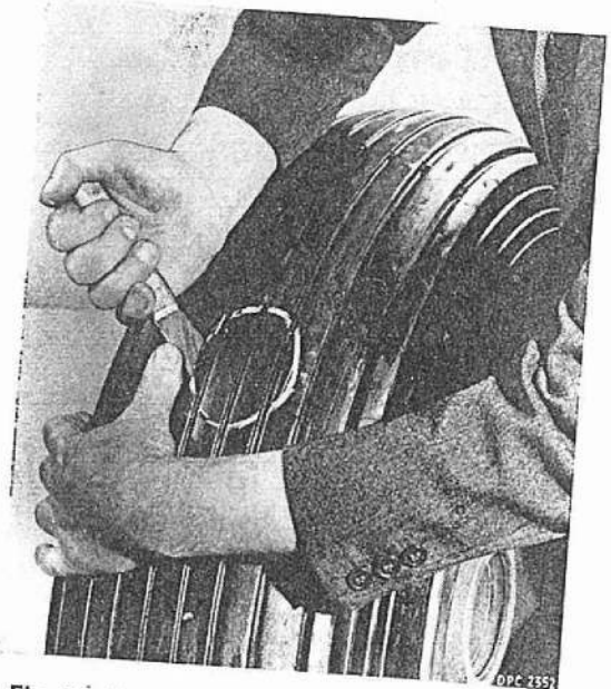
Fig. 2. Removal of damaged rubber—using a knife
