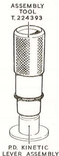
Fig. 14. Assembling the seals to the pressure drop kinetic lever assembly
