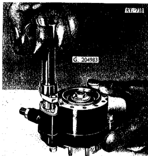
Fig. 2. Withdrawing the orifice body
