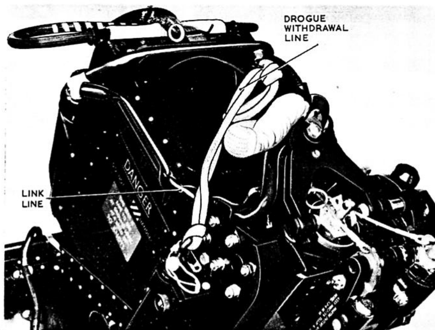
Fig. 12. Drogue withdrawal line
