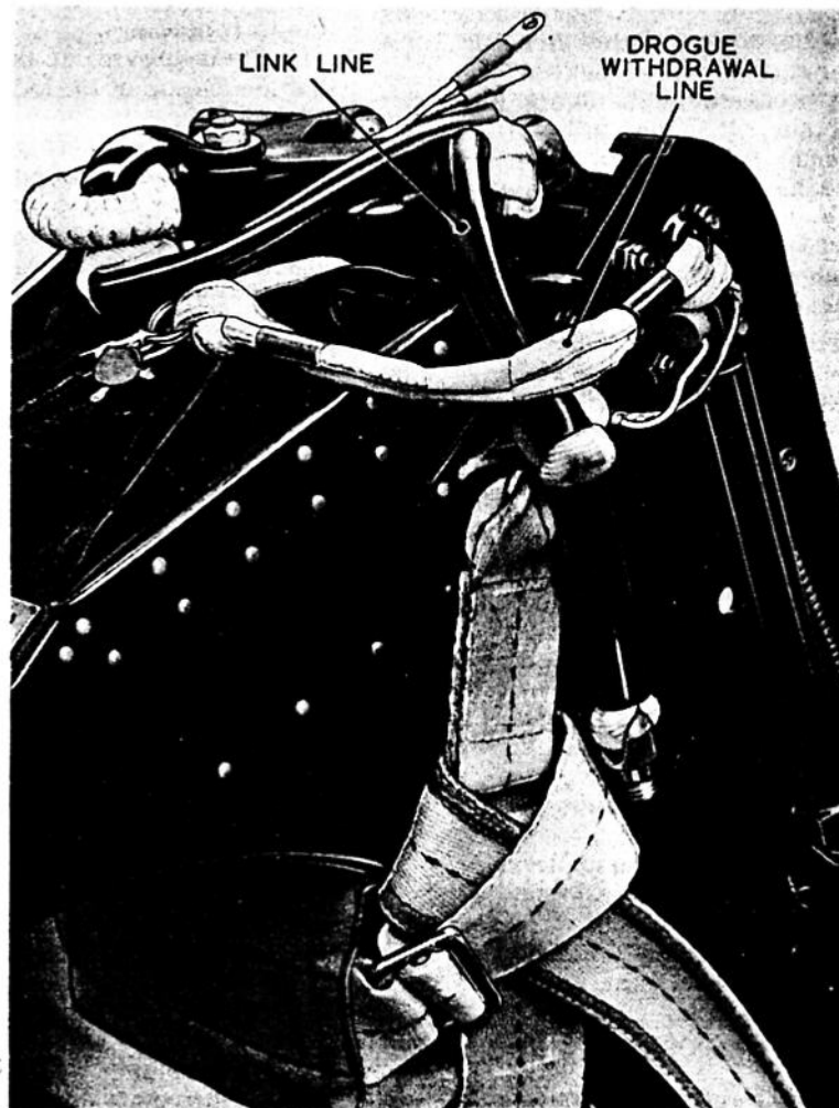
Fig. 13. Connecting drogue withdrawal line
