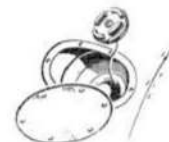
HYDRAULIC TANK FILLER CAP
