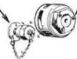
GROUND PRESSURE CONNECTION CABIN PRESSURE TEST CONNECTION AND GROUND PRESSURE CONNECTION ON THE PRESSURE BULKHEAD ACCESSIBLE THROUGH THE NOSE WHEEL WELL
