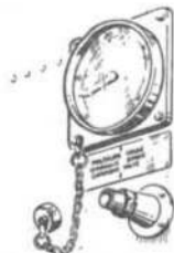
HYDRAULIC ACCUMULATOR AIR CHARGING VALVE AND PRESSURE GAUGE ON AFT FACE OF BOMB BAY FRONT BULKHEAD (PORT SIDE)
