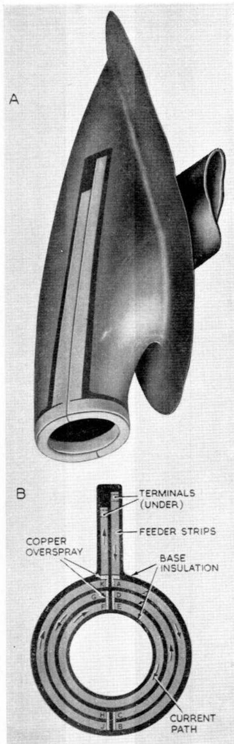
Fig. 5. Heater having remote terminals
