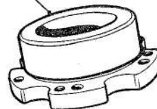
Fig. 35. Lower bearing housing location tool (reaming bearing)
