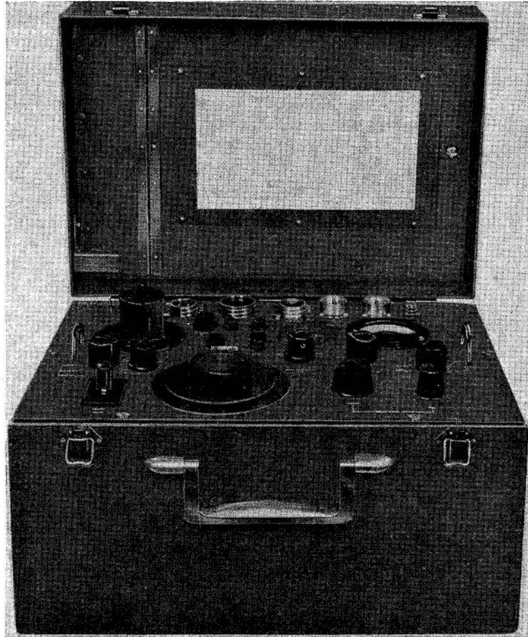
Fig. 1. Test equipment, ultra, Type Q2A8—control unit QC2A80
