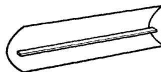
Fig.840.- Waveguide array feeding parabolic cylinder.
