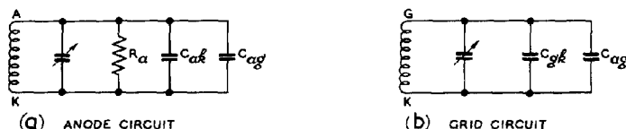
Fig. 398 - Common-cathode oscillator: effective tuned circuits.
