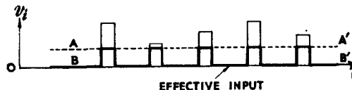
Fig. 486 - Limiting the amplitude of a succession of pulses.
