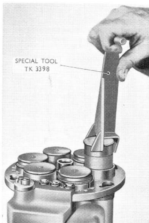
Fig. 5. Use of special tool for removing cartridges
