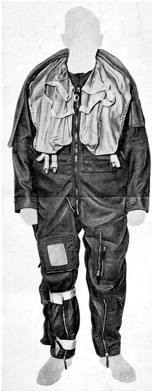
Fig. 3. Flying suit, Mk. 3—stole open to show lifting beackets
