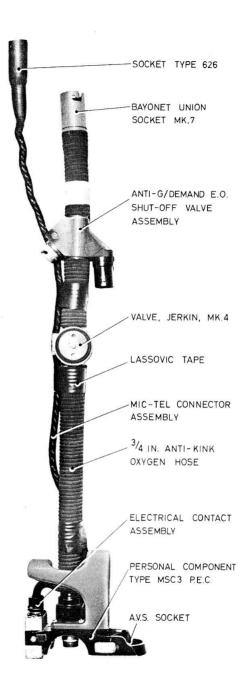
Fig. 5. Pressure jerkin hose assembly Mk. 6
