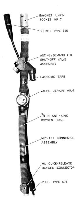
Fig. 7. Pressure jerkin hose assembly Mk. 9
