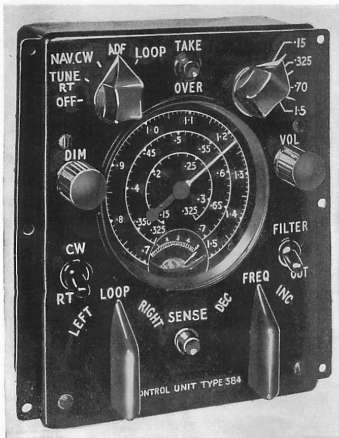
Fig. 1. Radio Compass (A.R.I. 5428) Control Unit.
