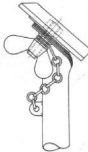
DETAIL "A" ATTACHMENT OF CONTROL COLUMN LOCKING BAR TO FUSELAGE SIDE.
