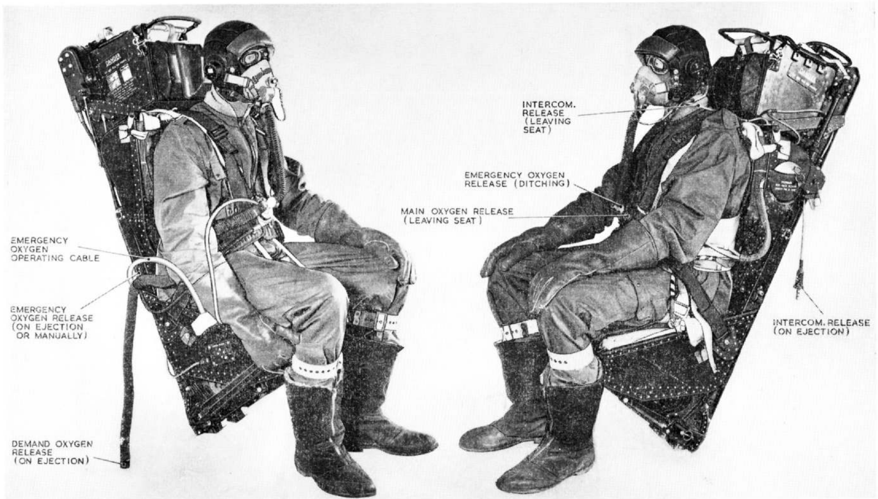
Fig. 2. Mk. 3A ejection seat (quick-release connections)
