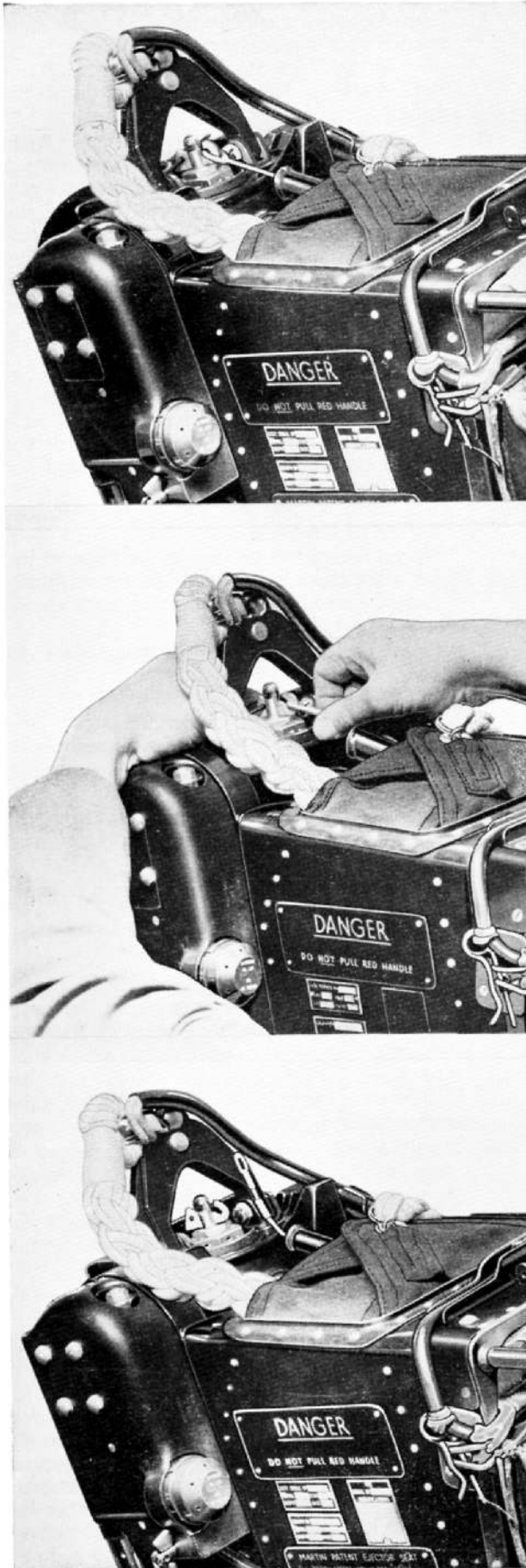
Fig. 2. Disconnecting firing cable from seat
