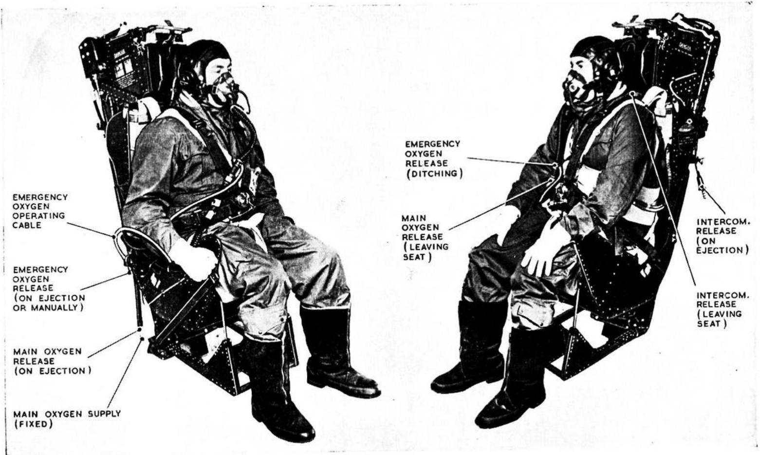
Fig. 2. Mk. 2A ejection seat (quick-release connections)
