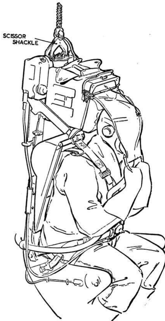
Fig. 5. Automatic operation—after ejection from aircraft (1)
