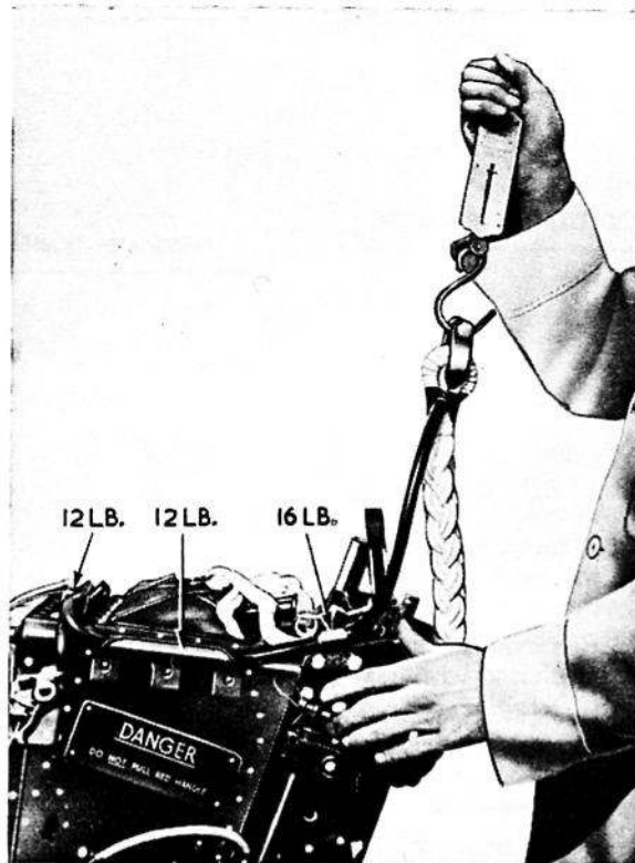
Fig. 18. Testing the lifting lines
