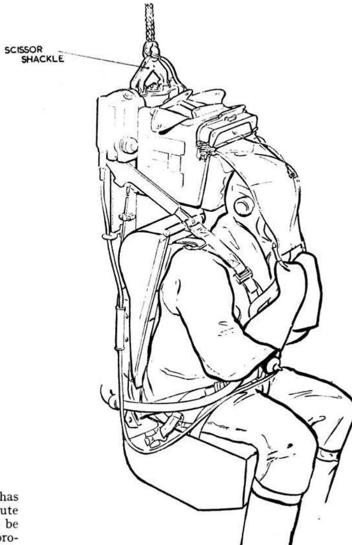
Fig. 6. Automatic operation—after ejection from aircraft (1)
