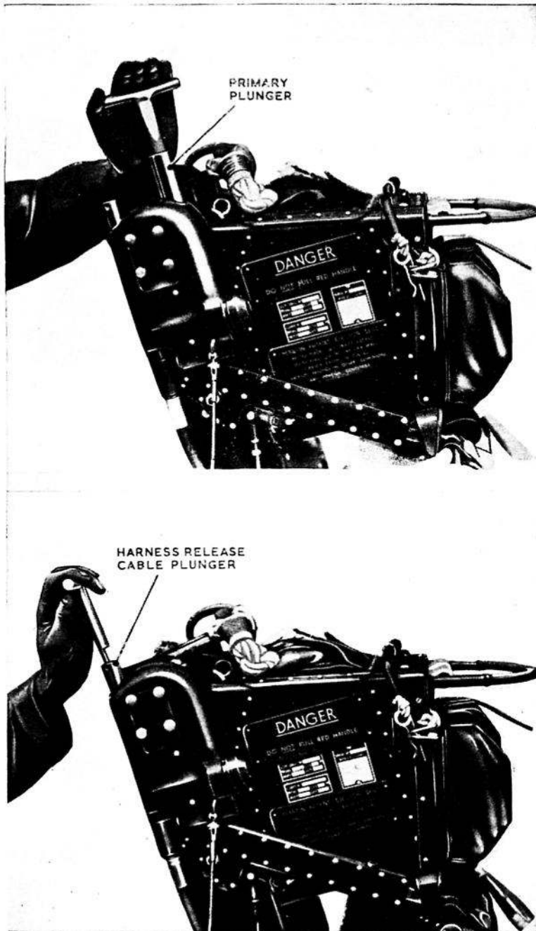
Fig. 18. Re-setting the barostatic time-release mechanism
