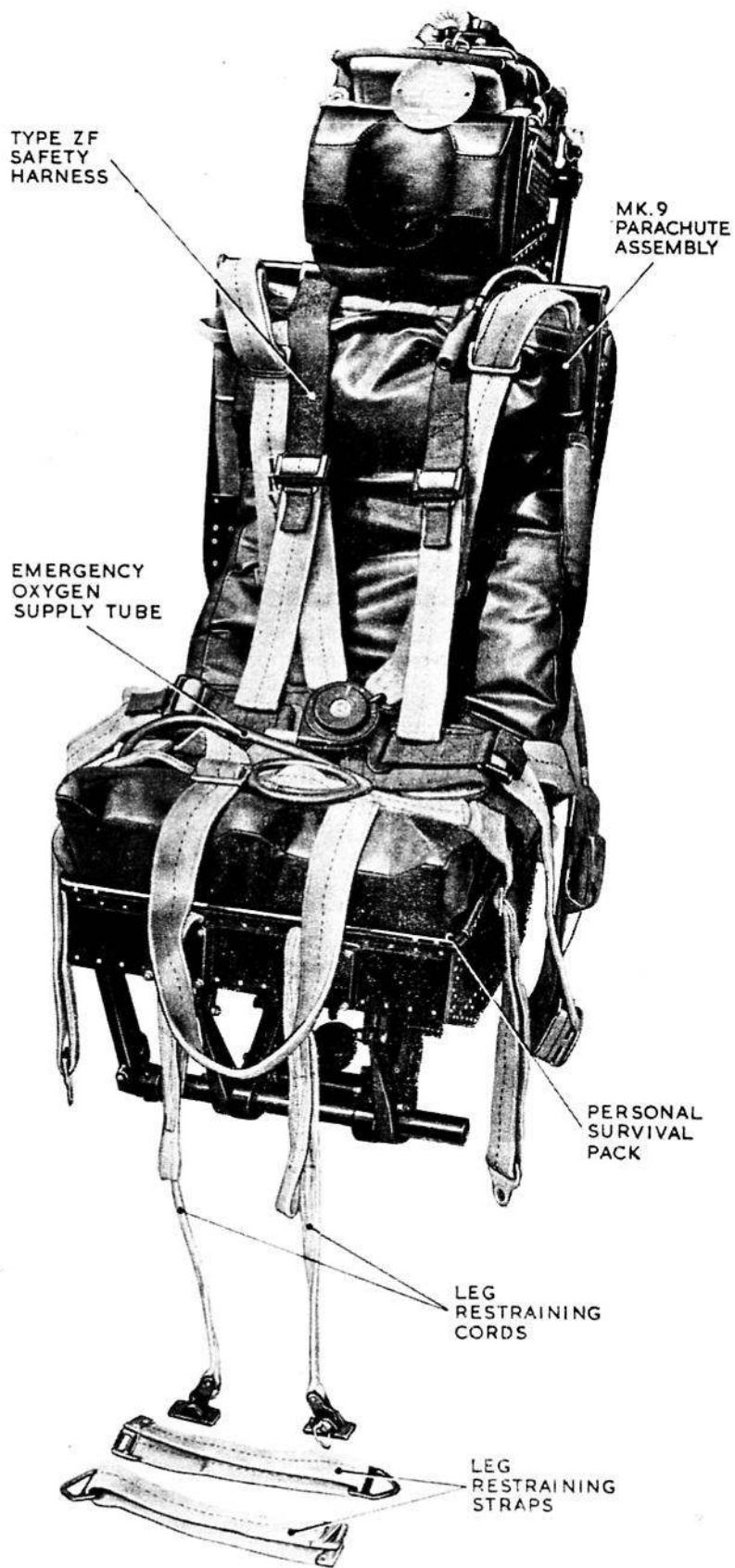
Fig. 1. Mk. 3B ejection seat emergency equipment
