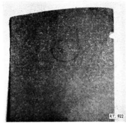
Fig. 4. Rotor blade—acceptable damage
