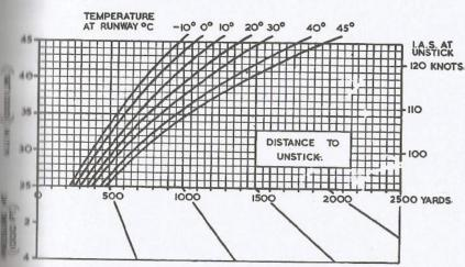
The example shows that in still air at a temperature of - 10°C. and a pressure height of 2,000 feet, the distance from wheels rolling to 50 feet, at an all-up weight of 35,000 lb. will be about 850 yards.
