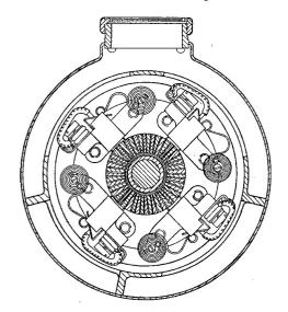
Fig. 1. Sectional view of brushgear
