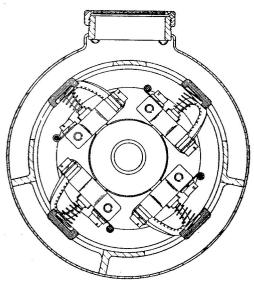
Fig. 3. Sectional view of brushgear (Type 201 shown)
