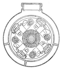
Fig. 2. Sectional view of brushgear
