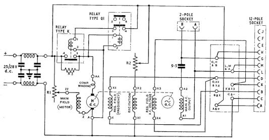
Fig. 4. Circuit diagram (Type 201 shown)
