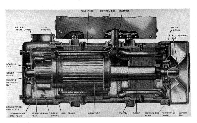
Fig. 2. Sectional view of inverter (Type 201 shown)
