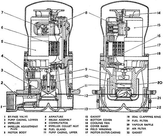
Fig. I. Sectional view of Mk. 3 pump
