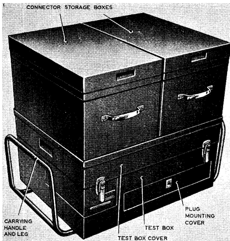
Fig. 3 Test set (early model)
