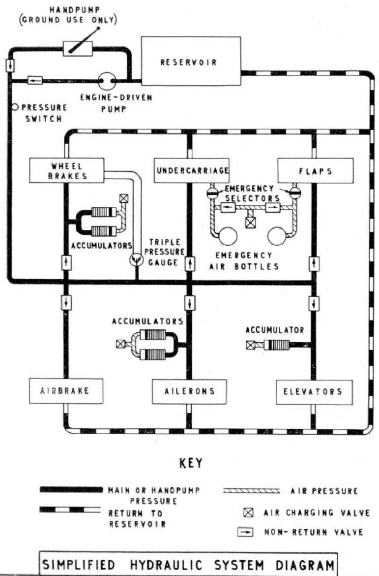
The main pressure is indicated by the central needle of the triple pressure gauge (26) at the forward end of the port shelf.
