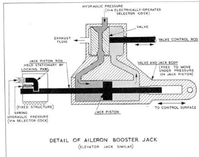
ailers, but to avoid excessively high stick forces the pawls automatically disengage and release the anchored jack piston rods, allowing them to slide freely with the movement of the jack bodies.
