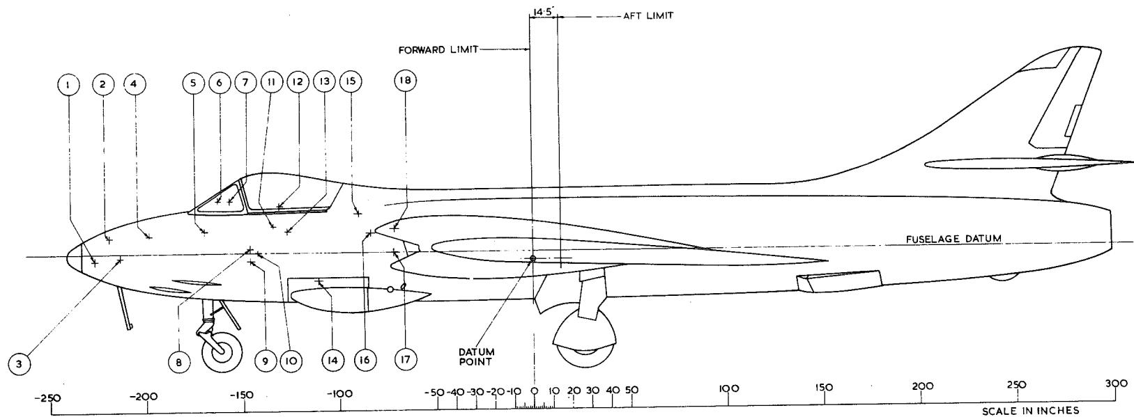
Fig.1 Loading and C.G. diagram
