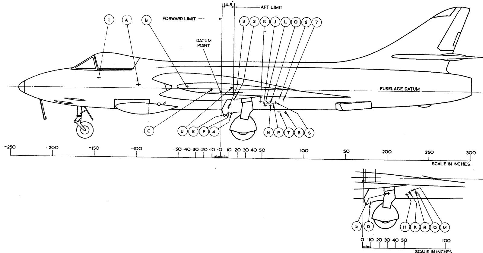
Fig.2 Loading and C.G. diagrams for Table 2 and 3 items.
