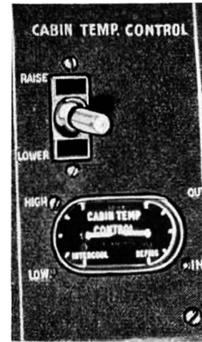
FIG 19 Cabin Temperature Control
