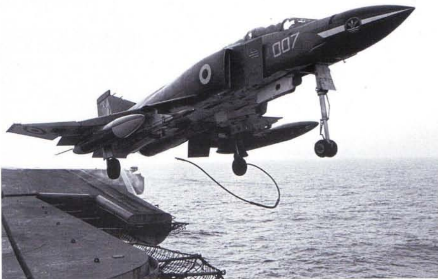
Left: A redundant strop falling into the sea after launching Phantom FG.1 coded 007 of 892 Squadron from the waist catapult on board HMS Ark Royal (MoD) Below: The power of the Phantom can be seen in this view of one of 892's aircraft taking off from RAF Luqa with full reheat (G.Mangion)
