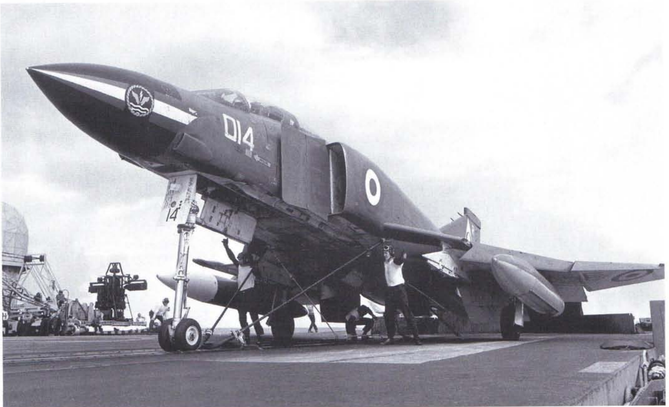
Strop fitted, oleo leg extended and ready for launch. A dramatic view of one of 892 Squadron's Phantom FG.1s on Ark Royal's port side catapult. (MoD)
