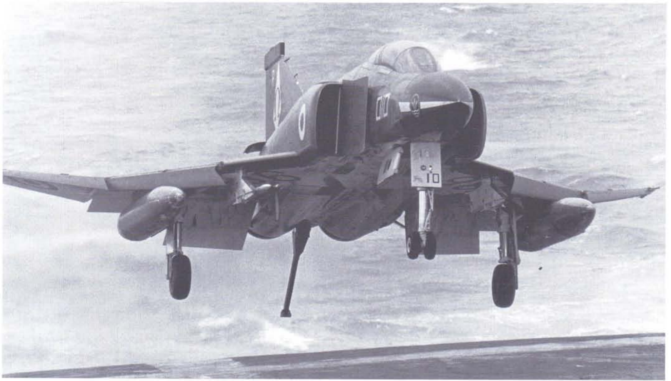
One of 892's Phantom FG.1s during the final cruise of Ark Royal seen over the ship's round down with the arrester hook lowered, flaps and leading edge slats extended, and about to take one of the arrester wires. (MoD)
