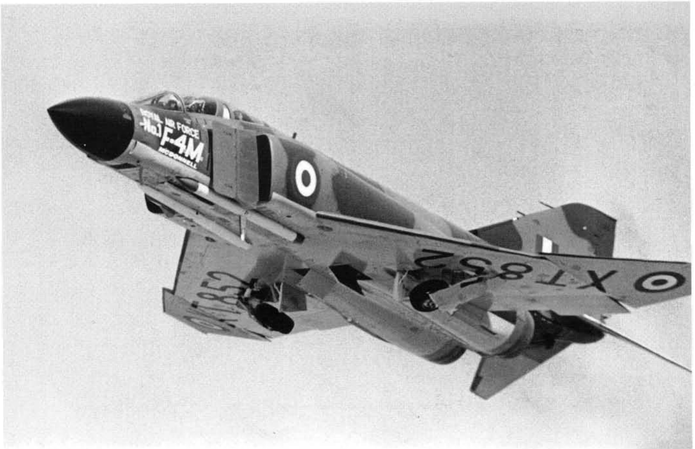
The first prototype of the F-4M for the RAF, XT852, seen tucking up the undercarriage during its flight testing in America. Two dummy Sparrow missiles on the forward fuselage stations house flight test instruments.
