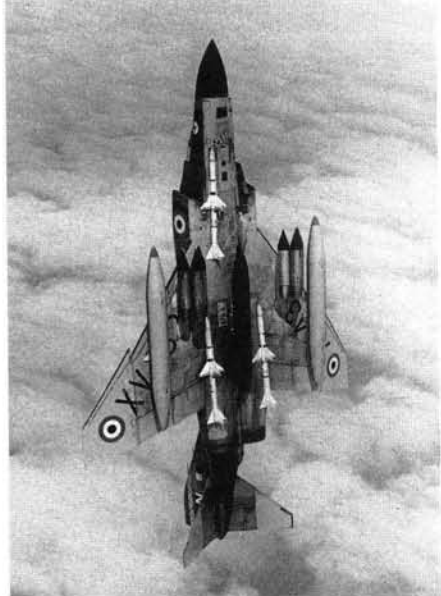
On the way up. A fully armed No. 6 Squadron Phantom FGR.2 in a vertical climb. Its rate of climb was 32,000 feet per minute.
